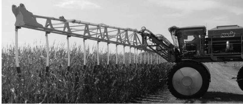
A cover crop interseeder can broadcast several hundred acres of cover crop seed in a day, allowing ag retailers and farmers to get cover crop seed established efficiently and early in the fall. Photo by Rob Myers, North Central SARE.
