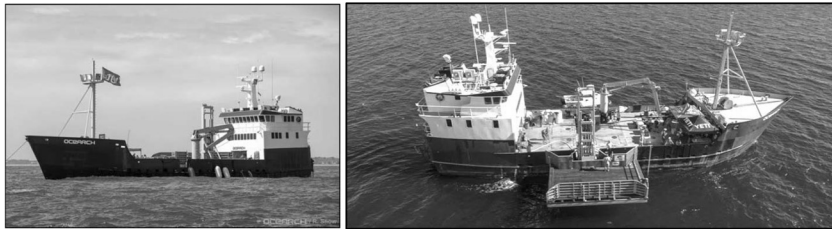
M/V OCEARCH , a specialized 130-foot research vessel designed to study large sharks. The hydraulic platform deployable off the starboard side of the ship can lift up to 75,000 pounds.
