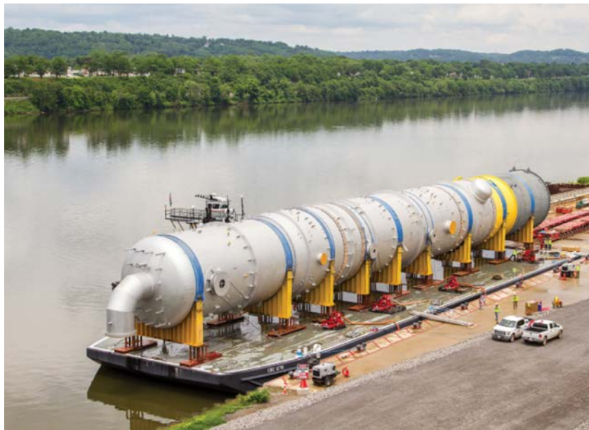
Figure 2—The M/V Big Eddie of Crosby Marine is seen at Monaca, PA (Mile 27.9 of the Ohio River) on May 30 with a deck barge carrying a large refiner vessel for the Shell Oil Corporation ethylene cracker plant under construction. Shown here are pumps used to level the barge for unloading, and the heavy-duty flatbed carrier to transport the equipment to the construction site. (Photo by Eric M. Johnson, Waterways Journal)
