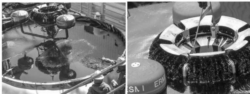
Figure 4. Helix skimmer during oil preload and testing.
