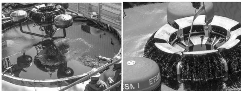
Figure 4. Helix skimmer during oil preload and testing.
