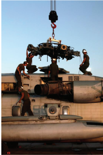
U.S. Marines with Marine Heavy Helicopter Squadron 462 perform maintenance on a CH-53E Super Stallion at Camp Bastion, Helmand province, Afghanistan, Oct. 14, 2013. The Marines removed the top rotor and prepared the aircraft for a replacement. (U.S. Marine Corps photo by Sgt. Gabriela Garcia/Released)
