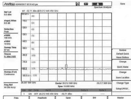
Figure 3.1-3 (P) Spectrum Photos 28 GHz - 100 kHz Res BW Site 8 at 2m AGL
