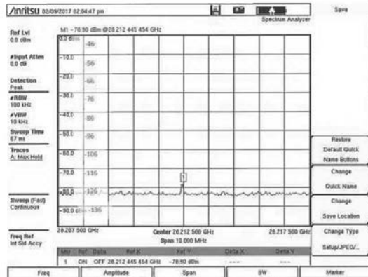
Figure 3.1-3 (L) Spectrum Photos 28 GHz - 100 kHz Res BW Site 6 at 2m AGL
