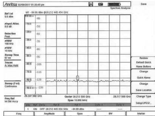
Figure 3.1-3 (H) Spectrum Photos 28 GHz - 100 kHz Res BW Site 4 at 2m AGL
