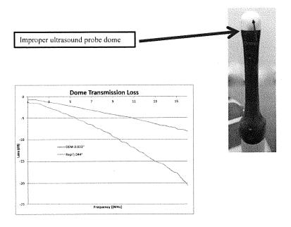
This improper repair could have resulted in delayed diagnosis or misdiagnosis as well as health conditions associated with a non-biocompatible material.
