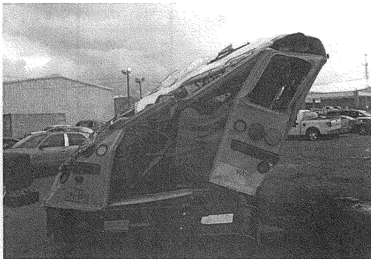
Figure 5. View of the rear of the HISD bus showing contact damage to the top left corner.
