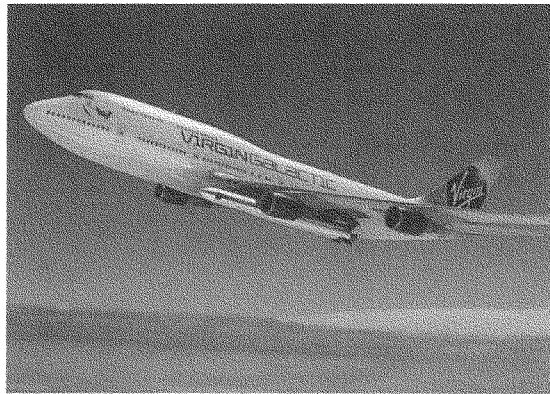
Figure 5: Modified Boeing 787-400 carrying the LauncherOne rocket
