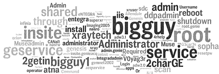
Figure 1: One medical device manufacturer had 35 CVEs and 125+ sets of exposed credentials. This word cloud, courtesy of Scott Erven, describes common default passwords from a single medical device manufacturer. Default passwords on cameras and other IoT devices enabled attackers to direct a tsunami of network traffic at Dyn. Similar default password risks exist for medical devices.
