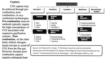
input to release the CO2 and regenerate the solvent, it results in significant reductions in overall plant efficiency and a substantial increase in cost. A third process, **oxy combustion**, requires expensive and energy intensive air separation units. While oxy systems hold promise, they are more experimental. Overall, while capture technologies exist, the new challenges associated with operating at a larger scale will not become clear until after full-scale deployment.
