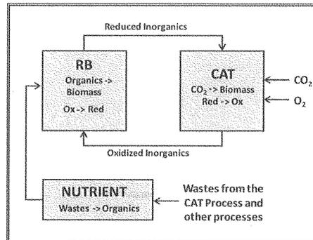
Figure B-2: Schematic of the CAT™ process.
