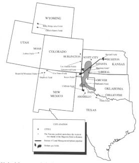
Figure 2.The United States crude helium supply system. Historically, the Hugoton and surrounding fields have been the principal sources of helium. Recently, natural gas fields in Wyoming with rich helium and other non-fuel content have become an increasingly important supply of helium, while potential new fields are located in the Four Corners area. SOURCE: U.S. Geological Survey 2006 Minerals Yearbook (Helium).
