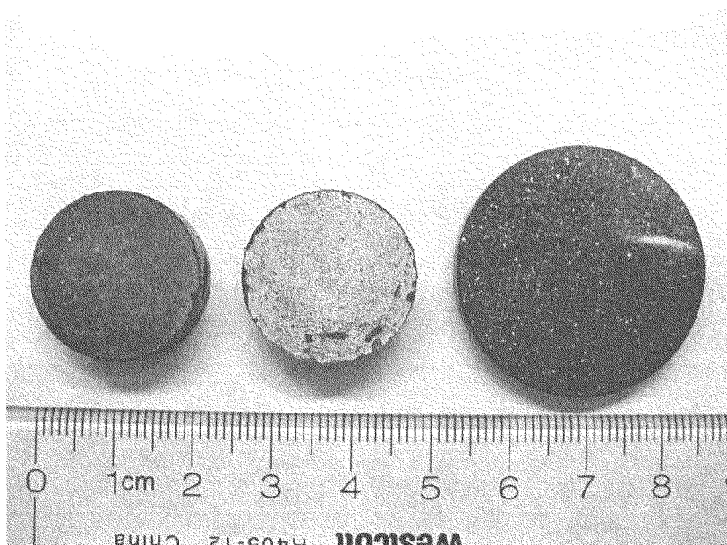
FIGURE CAPTION: The first and second \text{Nd}_2\text{Fe}_{14}\text{B} bonded permanent magnet prepared using the new process for making the neodymium master alloy.
