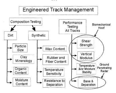
Figure 2: A chart of the tests which can be used to manage racing surfaces.
