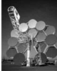
A solar **dish-engine** system is shaped much like large satellite dishes and covered with curved mirrors. The dish is programmed to always face the sun and focus that energy on a receiver at the dish's focal point, in much the same way that a satellite dish focuses radio waves on a tuner. The receiver is connected to a Stirling engine, which uses the thermal power generated by the focused solar energy to
