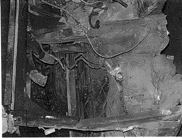
Fender Well Missing: Aluminum Body could Not withstand explosion turning into shrapnel
