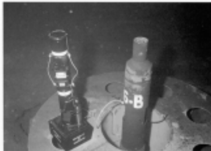
A COMC (Circulation Observation Moored Cables) sits in a seafloor burrhole, measuring seafloor fluid circulation processes that may affect earthquakes, sea level rise, and seafloor sediment composition.
