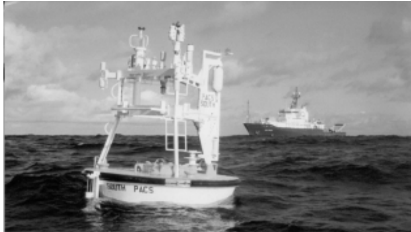
A WAVE moored surface buoy equipped with meteorological and hydrographic sensors is deployed in the eastern tropical Pacific Ocean from Scripps Institution of Oceanography's R/V Roger Revelle. Fixed in strategic ocean locations, surface and subsurface moored observatories (see this issue's special section) track oceanic processes and atmospheric interactions that influence Earth's climate.
