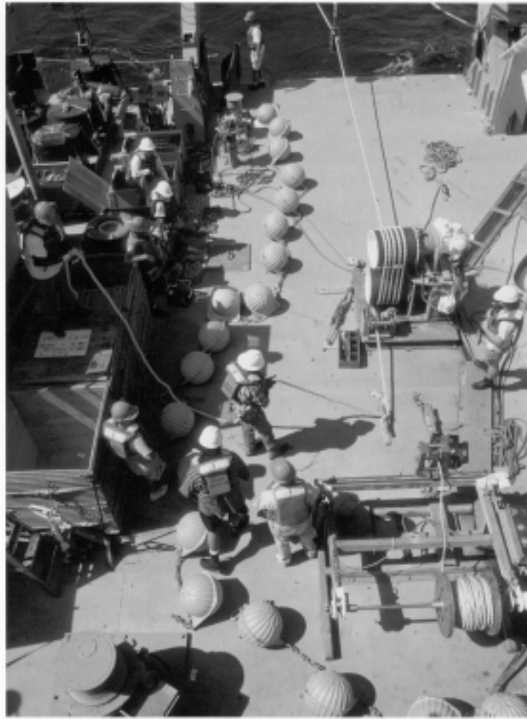
A long line of glass balls in yellow "hardhats" will provide flotation for a moored buoy observatory in the Pacific Ocean.
