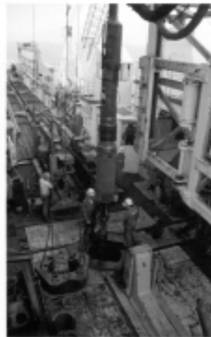
Aboard the ODP drill ship JOIDES Resolution, rough-seals junction at CORRS observatory in a long segmented drill pipe leading to a borehole in the seafloor.
