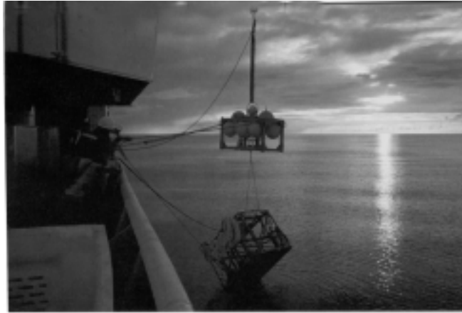
Thomas Thompson crew members prepare to submerge H2O's first "sensors" a package of instruments to record earth-quake-generated seismic waves.
