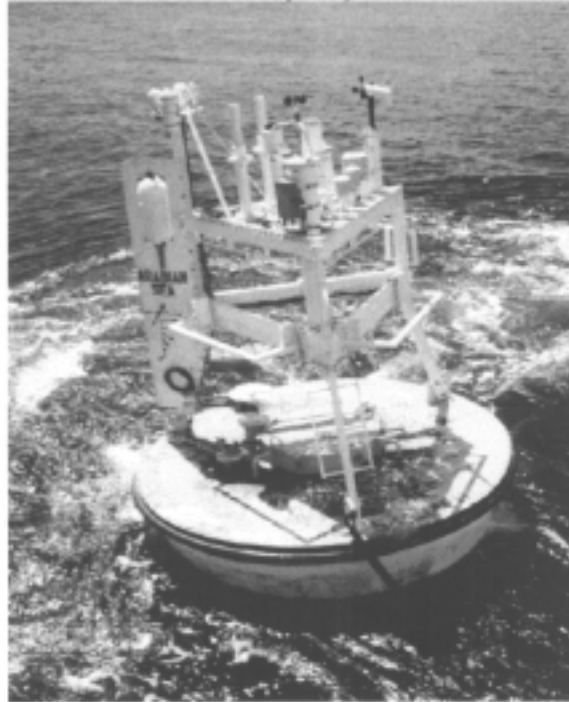
Figure 6. Surface buoy equipped with meteorological sensors to measure all the variables (wind velocity, air and sea temperature, rain, barometric pressure, relative humidity, incoming shortwave radiation, and incoming longwave radiation) needed to compute the air-sea exchanges of heat, freshwater, and momentum.
