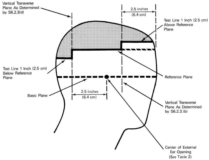
Note: Solid lines would correspond to the test line on a test helmet.
