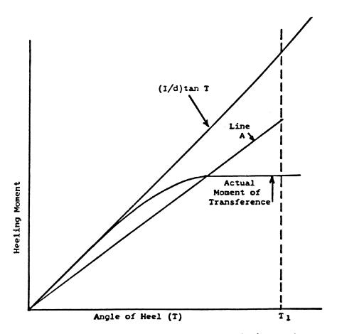
T<sub>1</sub> = the angle at which the deck edge is immersed or 28 degrees, whichever is smaller.
