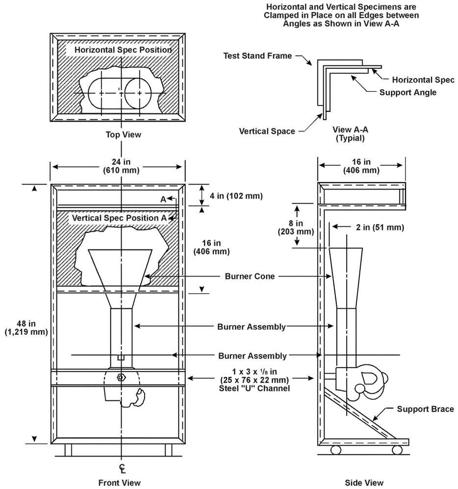
Figure 2: Calorimeter Bracket
