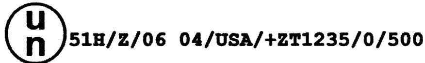
(iv) For a steel Large Salvage Packaging suitable for stacking; stacking load: 2,500 kg; maximum gross mass: 1,000 kg.
