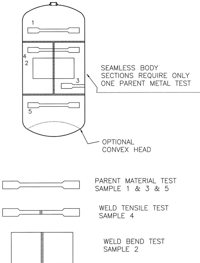
THIS FIGURE ILLUSTRATES THE PROPER TENSILE LOCATION FOR A 3 PIECE CYLINDER WITH THE HEADS HAVING STRAIGHT SIDEWALL.
