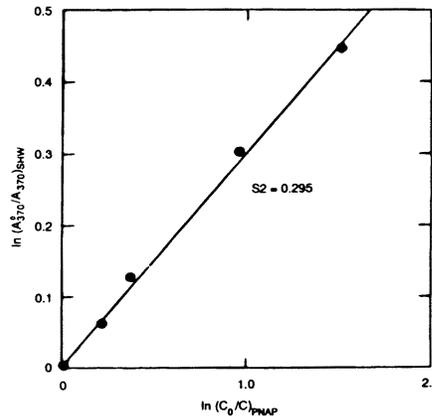
FIGURE 2—GRAPHIC DETERMINATION OF S2 = (K/K<sub>A</sub>) BASED ON EQUATION 12 UNDER PARAGRAPH (D)(1)(VII) OF THIS SECTION.
