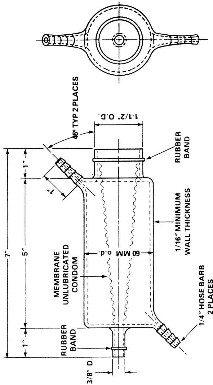
FIGURE 1 — SYNGYNA TEST CHAMBER
