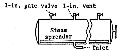
(1) Specifications. One 1-inch (2.5 centimeters) vent for every 5 feet (1.5 meters) of retort length equipped with a gate or plug cock valve and discharging to atmosphere; end vents not more than 2.5 feet (76 centimeters) from ends of retort. (2) Venting method. Vent valves should be wide open for at least 5 minutes and to at least 225 °F (107 °C), or at least 7 minutes and to at least 220 °F (104.5 °C).
