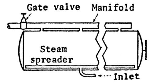
(1) Specifications. One 1-inch (2.5 centimeters) vent for every 5 feet (1.5 meters) of retort length; and vents not over 2.5 feet (76 centimeters) from ends of retort. Size of manifold—for retorts less than 15 feet (4.6 meters) in length, 2.5 inches (6.4 centimeters); for retorts 15 feet (4.6 meters) and over in length, 3 inches (7.6 centimeters).
