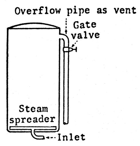
(1) Specifications. A 1.5-inch (3.8 centimeters) overflow pipe equipped with a 1.5-inch (3.8 centimeters) gate or plug cock valve and with not more than 6 feet (1.8 meters) of 1.5-inch (3.8 centimeters) pipe beyond the valve before break to the atmosphere or to a manifold header.
