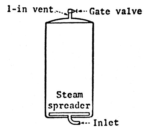
(1) Specifications. A 1-inch (2.5 centimeters) vent in lid or top side, equipped with a 1-inch (2.5 centimeters) gate or plug cock valve and discharging directly into the atmosphere or to a manifold header.
