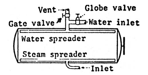
(1) Size of vent and vent valve. For relength, 2 inches (5.1 centimeters); for torts less than 15 feet (4.6 meters) in
