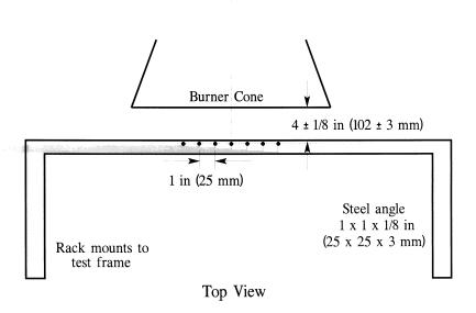
Figure 5 – Thermocouple Rake Position Relative to Burner Cone
