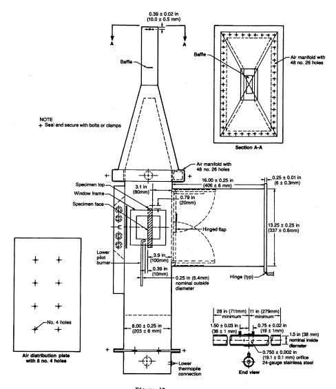
Rate of Heat Release Apparatus
