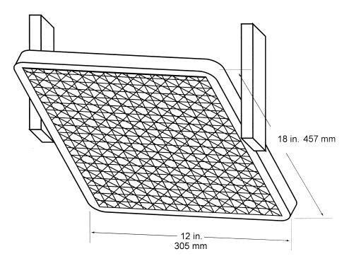
Figure 3b – Air Propane Radiant Panel
