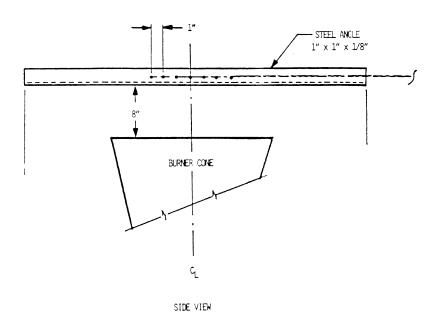
FIGURE 3. THERMOCOUPLE RAKE BRACKET
