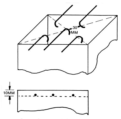
Figure 5. Thermocouple Position
