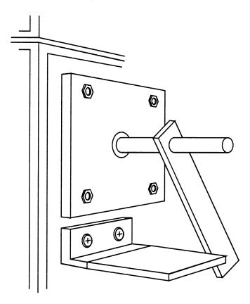
Figure 8 - Propane Burner Stop
