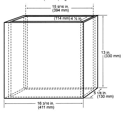
Figure 2 - Internal Chimney
