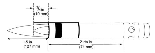
Figure 6 – Propane Pilot Burner
