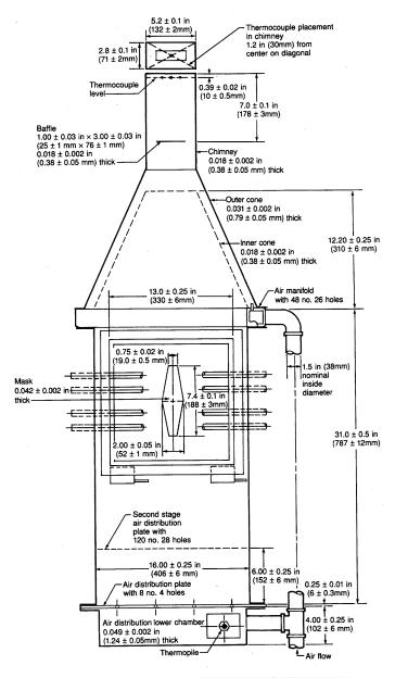
Figure 1A Rate of Heat Release Apparatus
