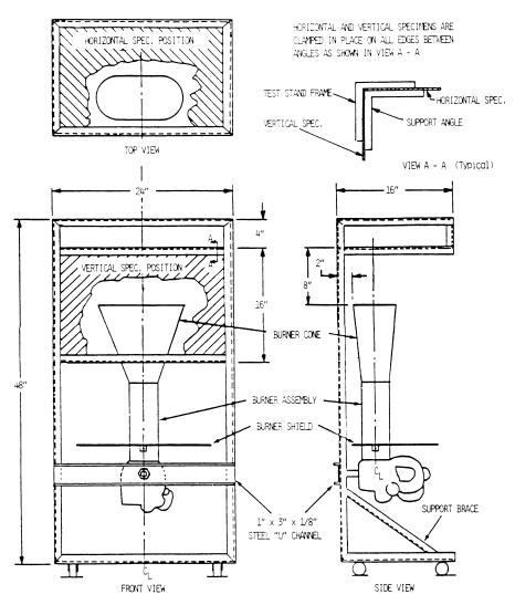
TEST STAND IS CONSTRUCTED WITH 1"  $\times$  1"  $\times$  1/8" STEEL ANGLES, ALL JOINTS WELDED SUPPORT ANGLES ARE 1"  $\times$  1"  $\times$  1/8" CUT TO FIT
