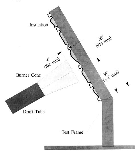
Figure 2 – Burnthrough Test Apparatus
