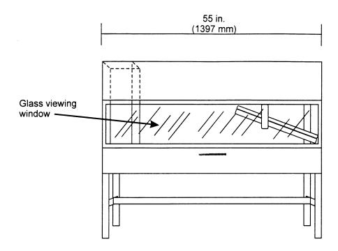
Figure 1 - Radiant Panel Test Chamber
