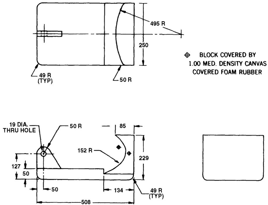
Figure 2.—Body Block for Lap Belt
