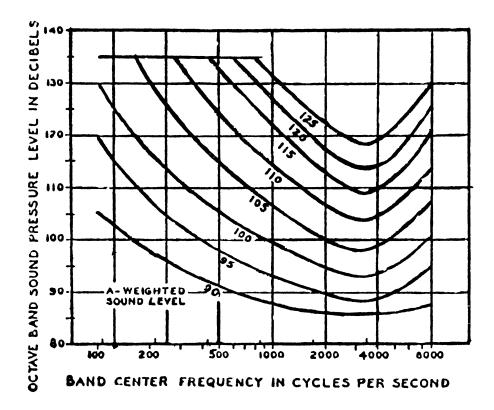
Equivalent sound level contours. Octave band sound pressure levels may be converted to the equivalent A-weighted sound level by plotting them on this graph and noting the A-weighted sound level corresponding to the point of highest penetration into the sound level contours. This equivalent A-
