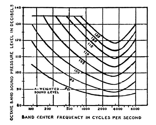
Equivalent sound level contours. Octave band sound pressure levels may be converted to the equivalent A-weighted sound level by plotting them on this graph and noting the A-weighted sound level corresponding to the point of highest penetration into the sound level contours. This equivalent Aweighted sound level, which may differ from the actual A-weighted sound level of the noise, is used to determine exposure limits from Table I.
