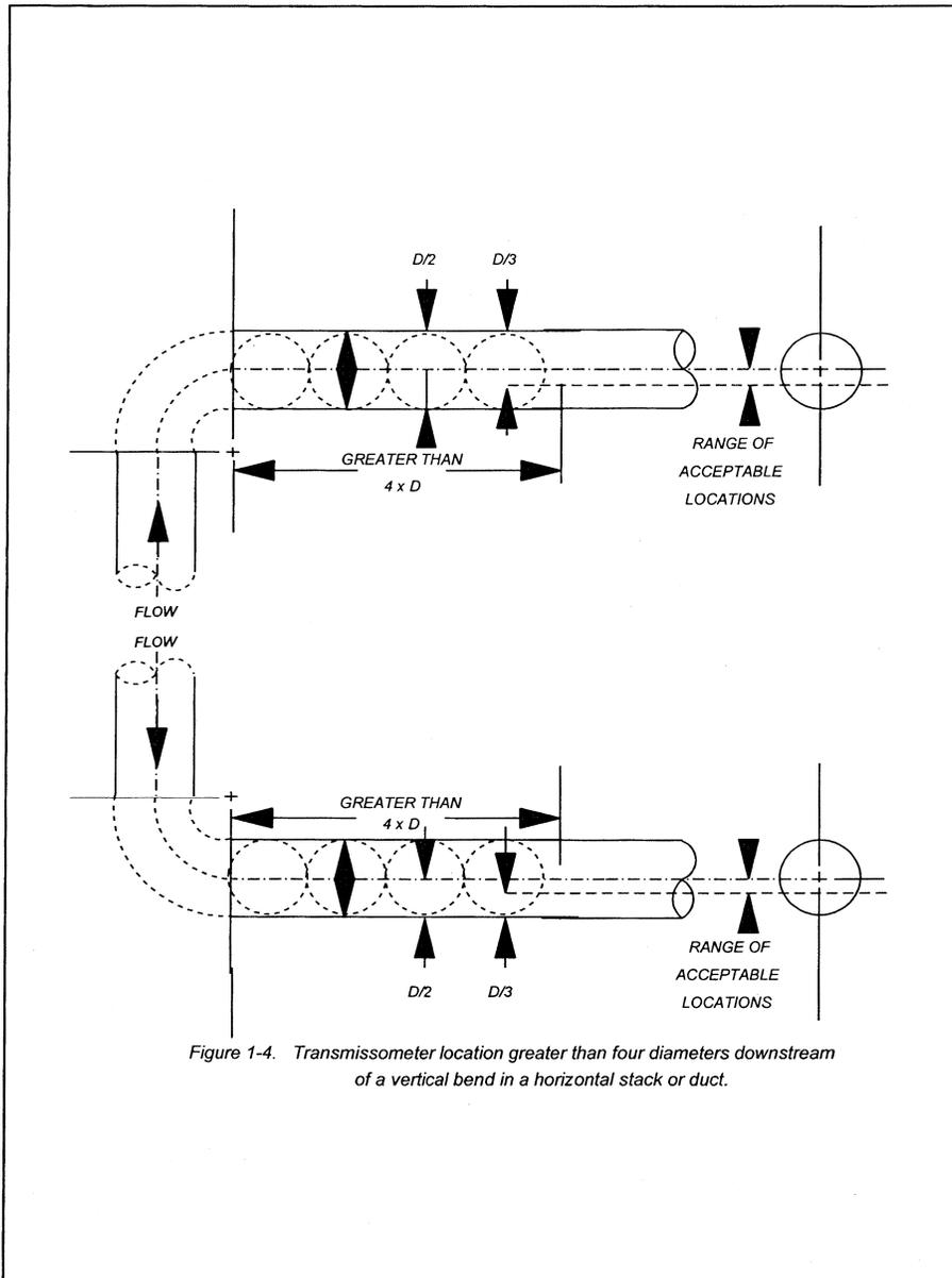
Figure 1-4. Transmissometer location greater than four diameters downstream of a vertical bend in a horizontal stack or duct.
