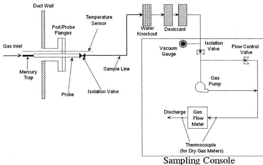
Figure 12B-1. Typical Sorbent Trap Monitoring System (only one trap and associated sampling system is illustrated).
