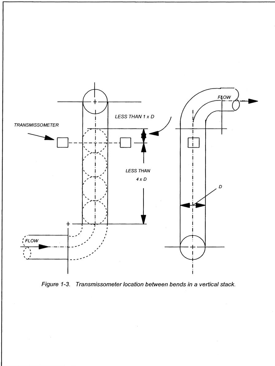
Figure 1-3. Transmissometer location between bends in a vertical stack.
