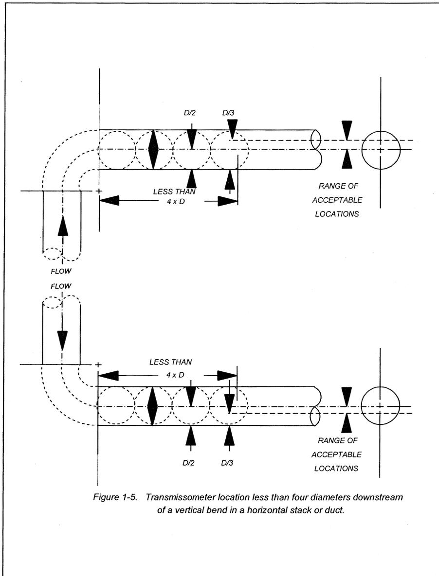
Figure 1-5. Transmissometer location less than four diameters downstream of a vertical bend in a horizontal stack or duct.
