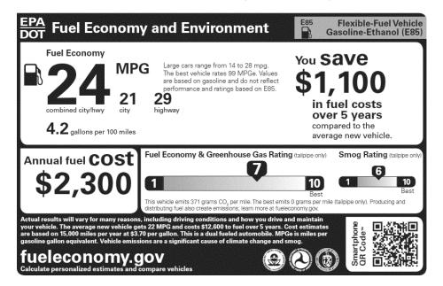
E. DUAL FUEL VEHICLE LABEL (ETHANOL/GASOLINE) WITH OPTIONAL DISPLAY OF DRIVING RANGE VALUES
