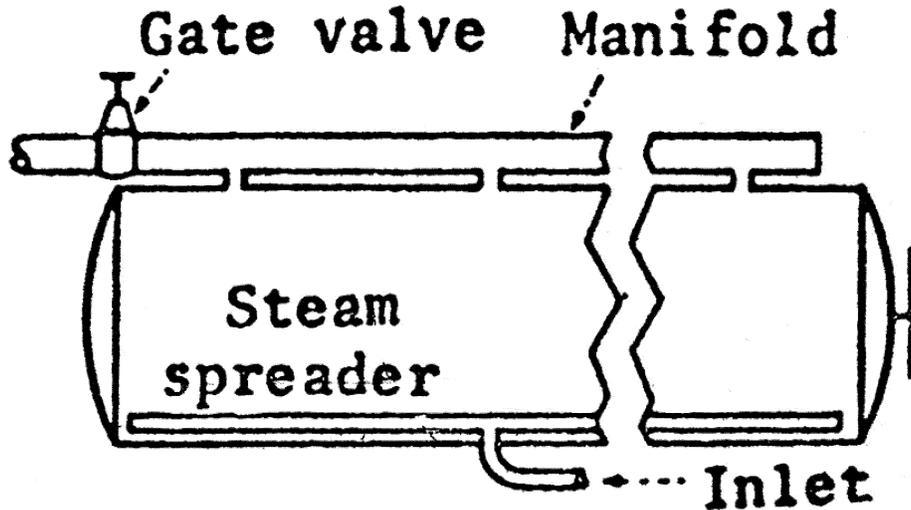
(1) *Specifications.* One 1-inch (2.5 centimeters) vent for every 5 feet (1.5 meters) of retort length; and vents not over 2.5 feet (76 centimeters) from ends of retort. Size of manifold—for retorts less than 15 feet (4.6 meters) in length,
