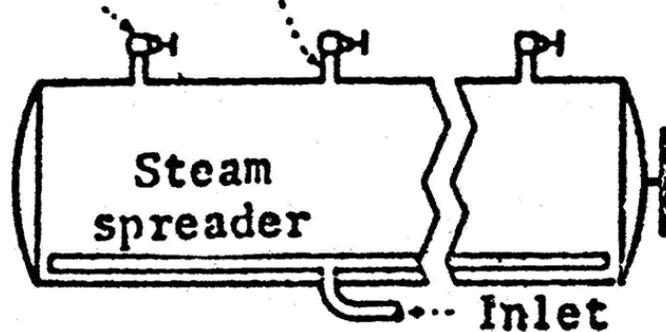
(1) *Specifications.* One 1-inch (2.5 centimeters) vent for every 5 feet (1.5 meters) of retort length equipped with a gate or plug cock valve and discharging to atmosphere; end vents not more than 2.5 feet (76 centimeters) from ends of retort.
