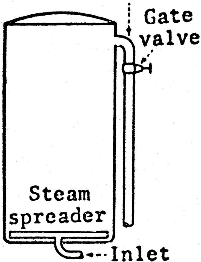
(1) *Specifications.* A 1.5-inch (3.8 centimeters) overflow pipe equipped with a 1.5-inch (3.8 centimeters) gate or plug cock valve and with not more than 6 feet (1.8 meters) of 1.5-inch (3.8 centimeters) pipe beyond the valve before break to the atmosphere or to a manifold header.
