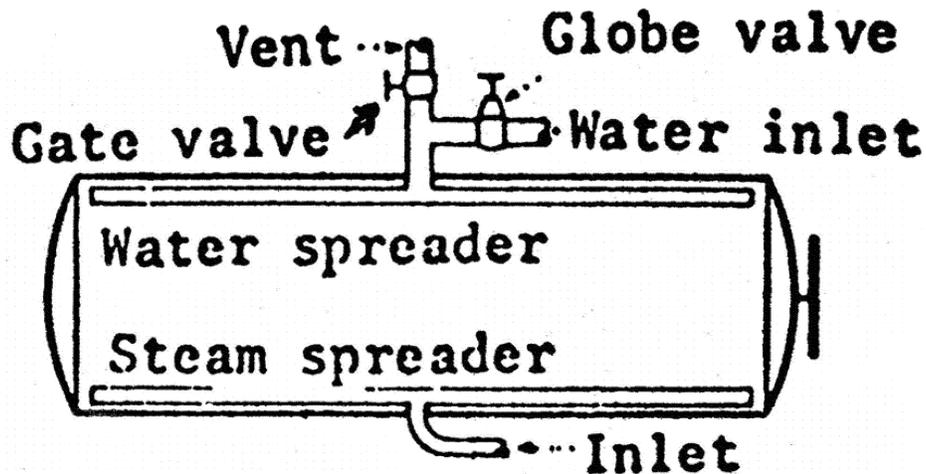
(1) *Size of vent and vent valve.* For retorts less than 15 feet (4.6 meters) in length, 2 inches (5.1 centimeters); for retorts 15 feet (4.6 meters) and over in length, 2.5 inches (6.4 centimeters).
