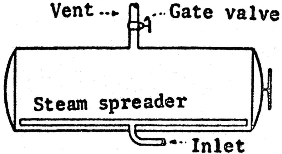
(1) *Specifications.* A 2.5-inch (6.4 centimeters) vent equipped with a 2.5-inch (6.4 centimeters) gate or plug cock valve and located within 2 feet (61 centimeters) of the center of the retort.
