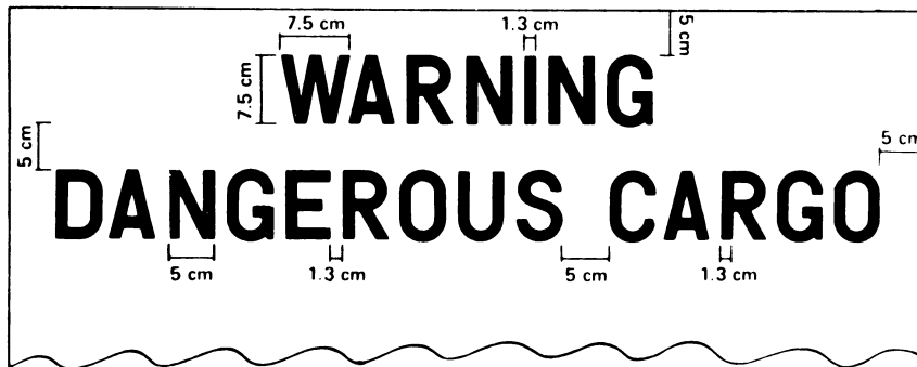
Figure 1 - Minimum Dimensions for Warning Sign
