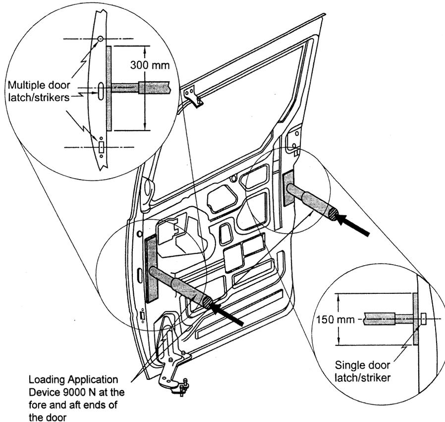
**FIGURE 10 – Sliding Door Full Vehicle Test Procedure**
