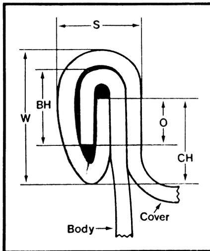
(b) *Seamscope or seam projector.* Required measurements of the seam include thickness, body hook, and overlap. Seam thickness shall be obtained by micrometer. For cylindrical containers, at least two locations, excluding the side seam juncture, shall be used to obtain the required measurements.
