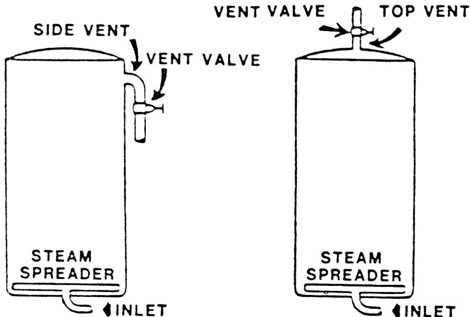
*Specifications (Figure 6 or 7):* A 1 inch (2.5 cm) vent in lid or top side, equipped with a gate, plug cock, or other full-flow valve and discharging directly into the atmosphere or to a manifold header.
