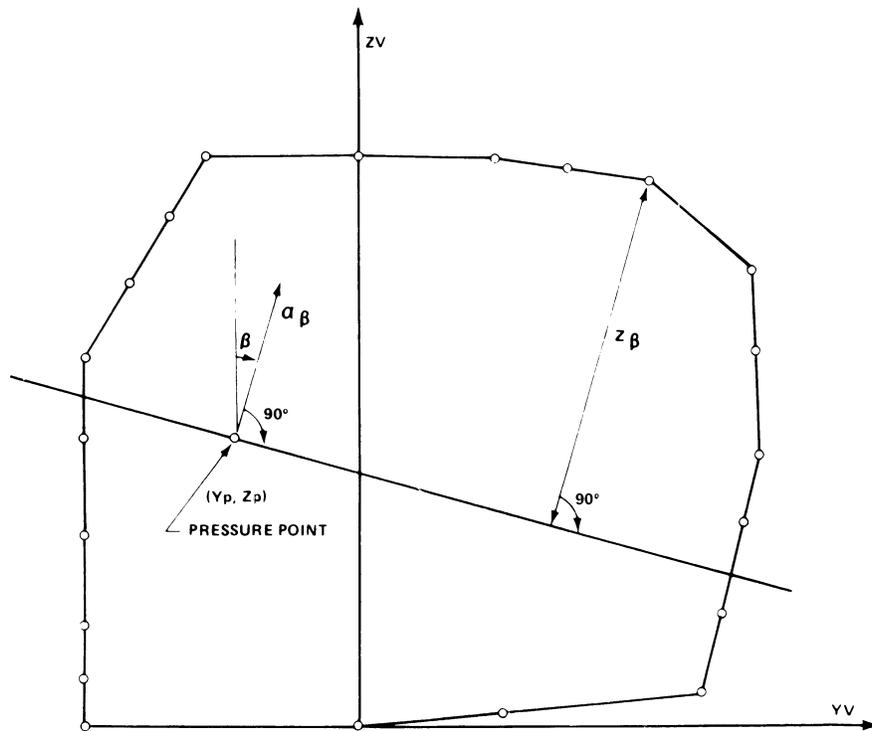
NOTE: LARGEST LIQUID HEIGHT ABOVE THE POINT WHERE THE PRESSURE IS DETERMINED =  $Z_{\beta}$
