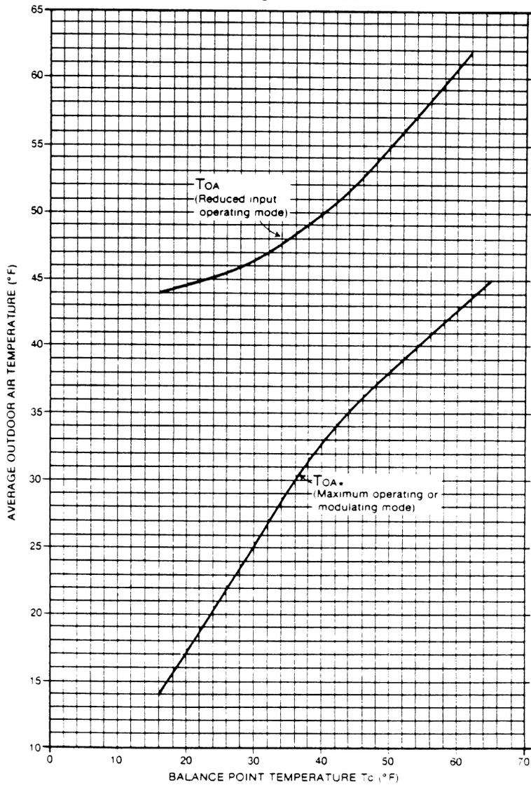
This figure is based on 4500 degree-days and 15°F outdoor design temperature
