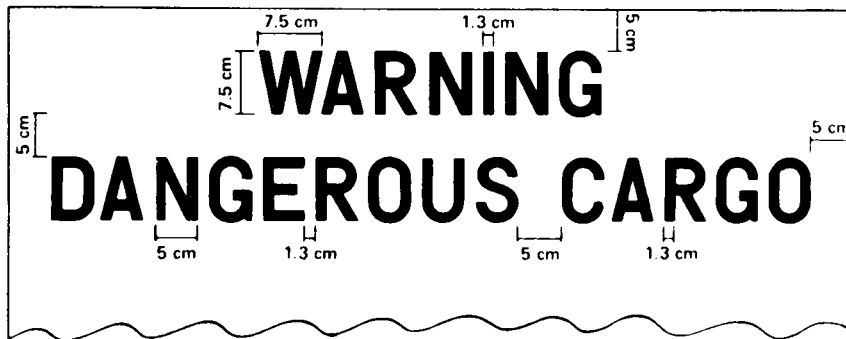
Figure 1 - Minimum Dimensions for Warning Sign
