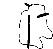
Fiber protrusion <5:1 Aspect Ratio
