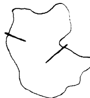
Fiber protrusion <0.5 micrometer
