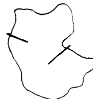
Fiber protrusion <0.5 micrometer
