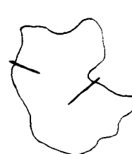
Fiber protrusion <0.5 micrometer
