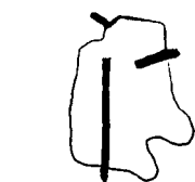
Fiber protrusion <5:1 Aspect Ratio
