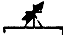
Locks making preparation, probably be ready in 10 minutes or less; you may approach with caution, prepared to tie up or enter on right-hand side on signal
