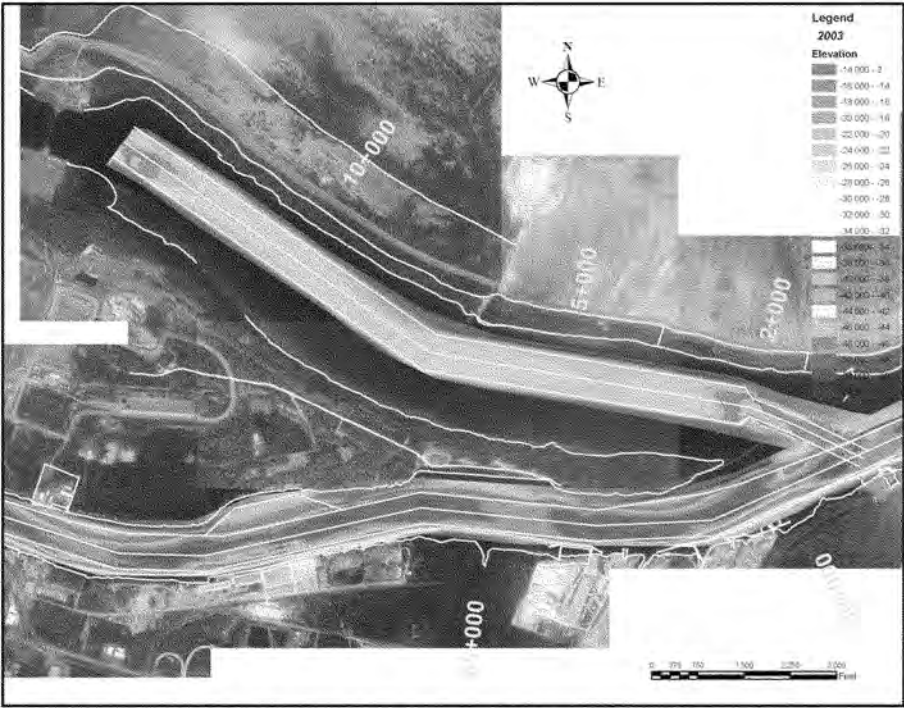
Figure 7-62 Sediment Basin 2003 Before Dredging Surface.
