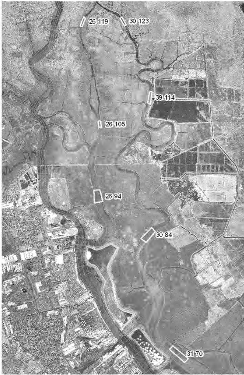
Figure 4: EFDC Grid Cell Locations Examined for Impacts to Tidal Fluctuations
