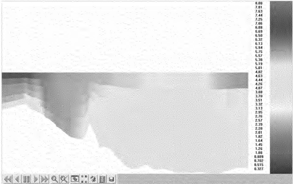
27. Figure B.18. Snapshot of 1-day averaged D.O. Dynamics (August 10, 1997) in vertical plane of Upper Harbor: Existing bathymetry
