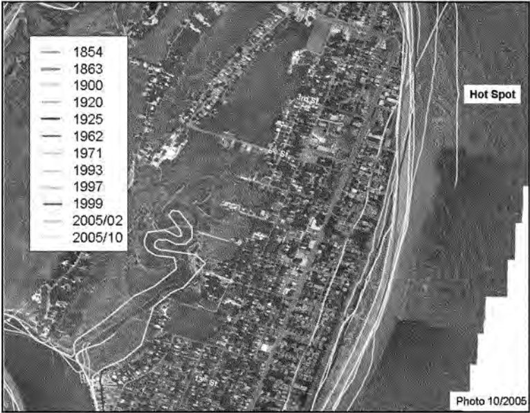
Figure 2-5. Historical shoreline positions along the central portion of Tybee Island in the vicinity of the hot spot.
