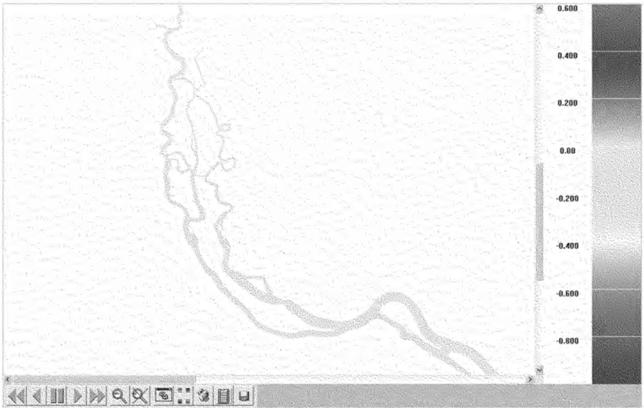
42. Figure A4.12. Changes in D.O. 5 th %ile distribution along surface layer: 2 ft deepening
