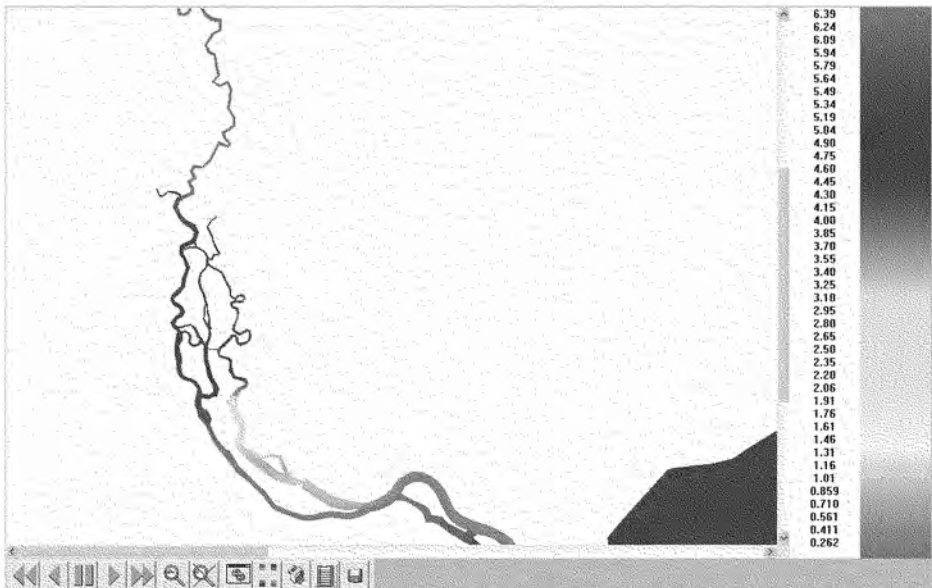
12. Figure B.3. Minimum D.O. distribution along surface layer within the analyzed period of May 1 - October 30, 1997: Existing bathymetry
