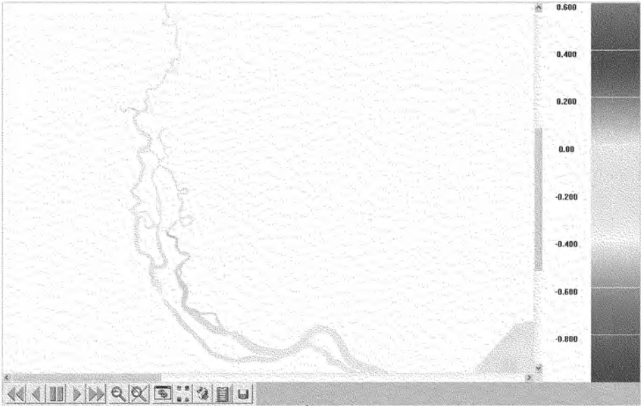
38. Figure B3.8. Changes in D.O. 95 th %ile distribution along bottom layer: 3 ft deepening
