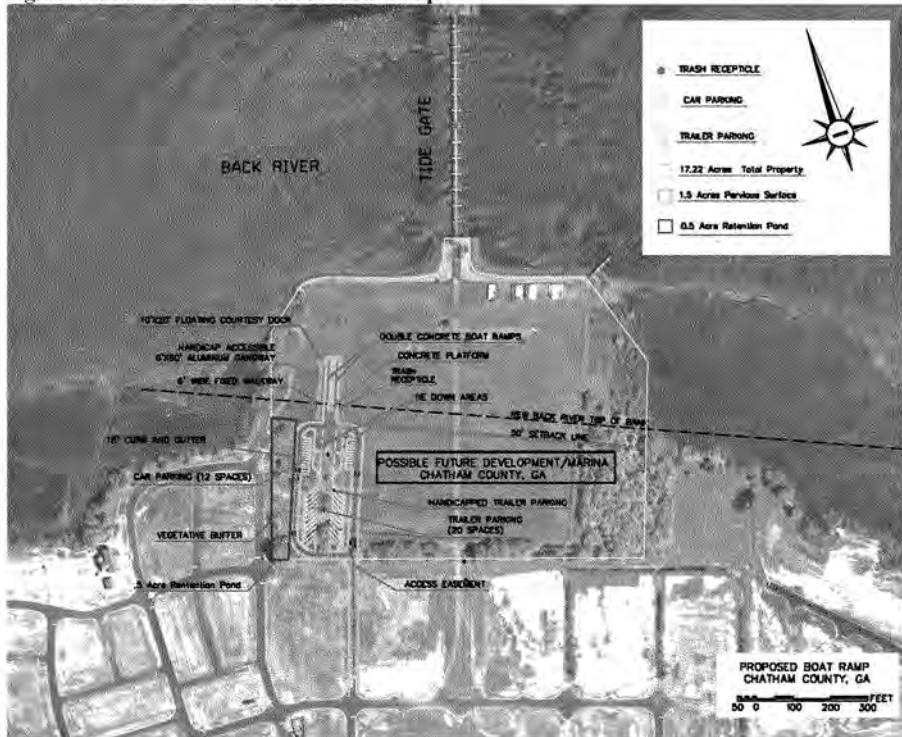
Figure 8.1.4-2: Hutchinson Island Boat Ramp
