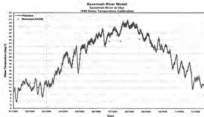
Figure 7 1999 Stream Temperature Calibration at Clio
