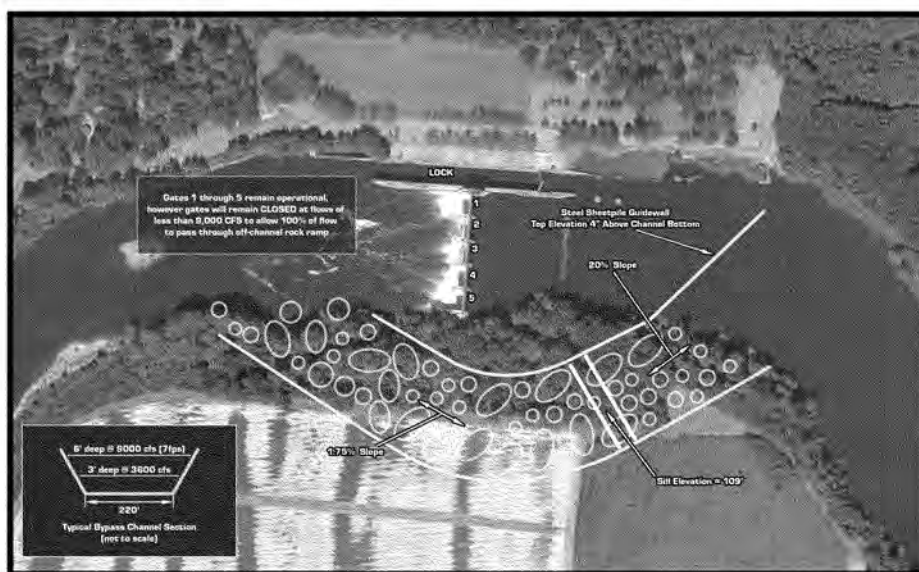
Figure 5-52. Conceptual design of off-channel rock ramp.
