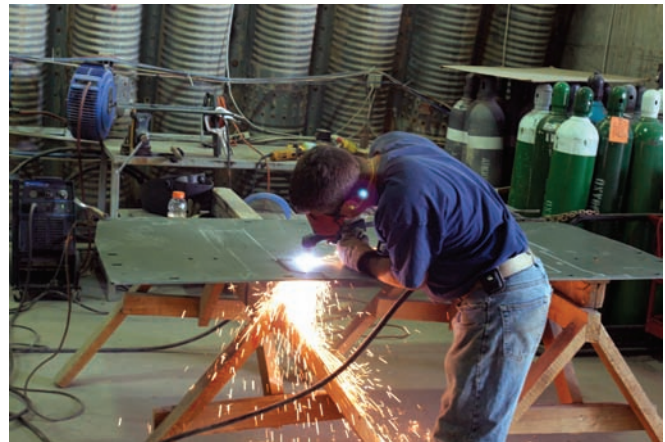
A civilian employee, who works to upgrade the Humvee A2s, prepares a piece of armor that will be used to further protect Marine vehicles against insurgent attacks.
