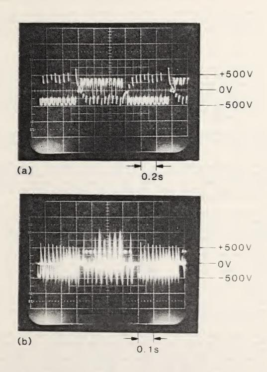
Figure 2. Photographs of two examples [(a) and (b)] of output waveform of device under test as measured using an oscilloscope
