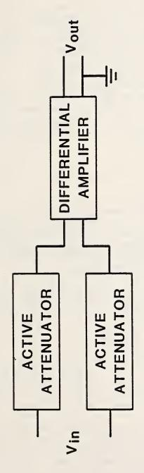
Figure 8. Block diagram of differential active attenuator
